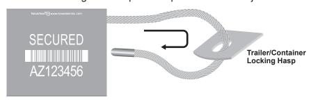
3. Pass the cable through the lock body until it exits the lock body; pull the cable tight to remove all slack on the hasp side.
