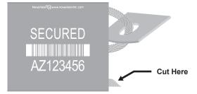
6. To remove cable, cut here with cable cutter.
