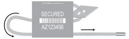
5. After removing all slack from the loops and lock assembly, cut off the free cable protruding from the lock body as close as possible to the lock.
