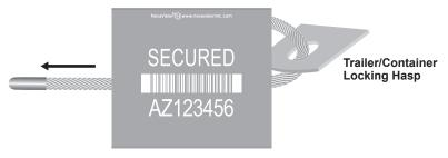
4. Reinsert the free end of the cable into the lock until it exits the lock body; pull cable tight to remove all slack from the second loop.
