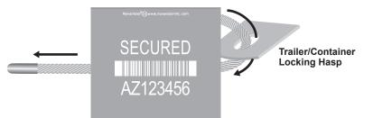
4. Reinsert the free end of the cable into the lock until it exits the lock body; pull cable tight to remove all slack from the second loop.
