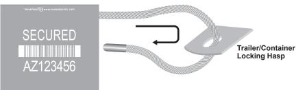
3. Pass the cable through the lock body until it exits the lock body; pull the cable tight to remove all slack on the hasp side.
