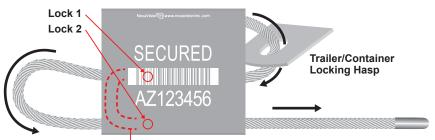
Cable Loop position when cable is fully tightened
