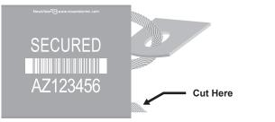
6. To remove cable, cut here with cable cutter.
