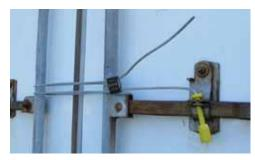
• Thread Cable into Cable Lock, pull taught to remove any slack.
