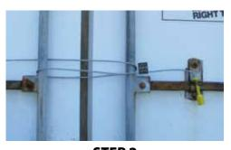
• Weave Cable through locking bars. Create a figure-eight for additional security.
