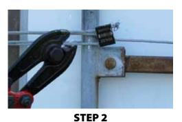
• Use Bolt Cutters or Cable Cutters to remove Cable Seal. Cut on fixed end near lock to prevent reuse.
