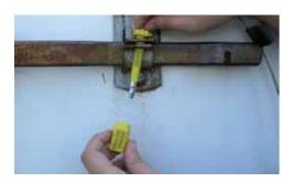
• Separate Bolt Seal from Lock, thread through latch hole and lock together
