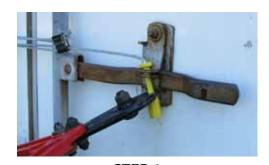
• Use Bolt Cutters to remove Bolt Seal. Use caution as bolt may come off at high speed.
