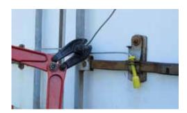
• Use Bolt Cutters or Cable Cutters to remove any excess cable. This prevents any reuse.
